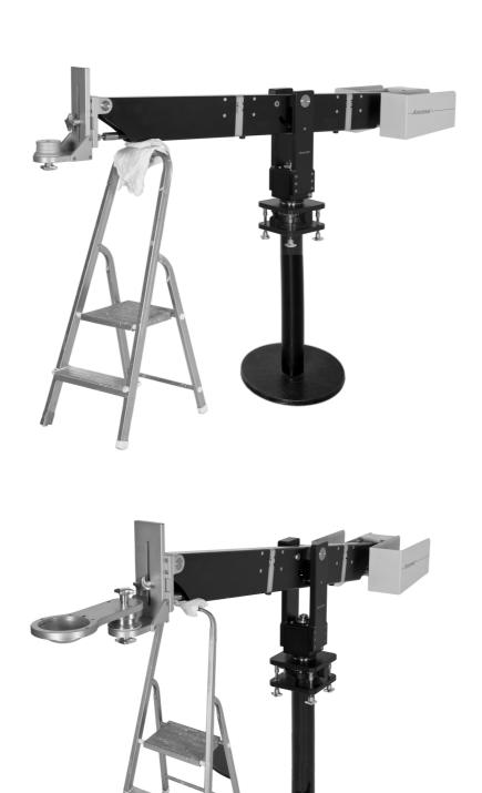
Balance the arm by putting some weight in the bucket, but maintain downward force on the support in the front end.
