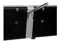
Once the dots are properly aligned, tighten the hammer bolt with the Swiss punch in the close direction, being careful not to over tighten. Warning, over-tightening may cause damage to the equipment.
