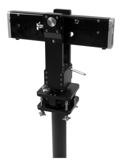
Place the fulcrum onto the leveling-head and turn the wheel in the fulcrum clockwise and tighten the tie down bolt with the Swiss punch.
